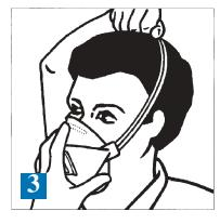
3. Cup respirator under chin. Ensure the two straps are seperated and pull the straps over the head.
