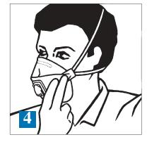
4. Locate the lower strap below the ears and the upper strap accross the crown of the head. Adjust top and bottom panels for a comfortable fit.
