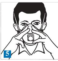
5. Using both hands, mould noseclip to the shape of the lower part of the nose.
