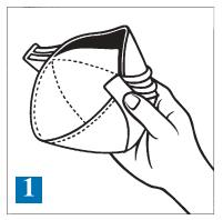
1. Noseclip is located in top panel. Preform noseclip by gently bending at centre
