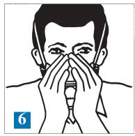
If you cannot achieve a proper fit do not enter contaminated area. See your supervisor. **6.** The seal of the respirator on the face should be fit-checked prior to wearing in the work area.
