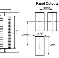
Note: 1. Recommended panel thickness is 1 to 8 mm.
