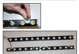
1) Position 'tab' end of first powerwhite module by input wires/driver. (<u>Do not connect power</u> to entry cable before completing steps 2-6)
