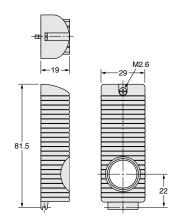
Note: 1 .The cover is provided with a rubber bushing and cap to prevent the cable from being pulled out in vertical direction.
