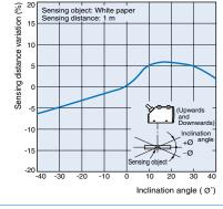
Sensing Object Angle (Left and Right)
