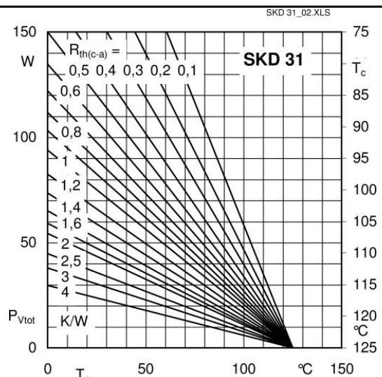
Fig. 3R Power dissipation vs. case temperature
