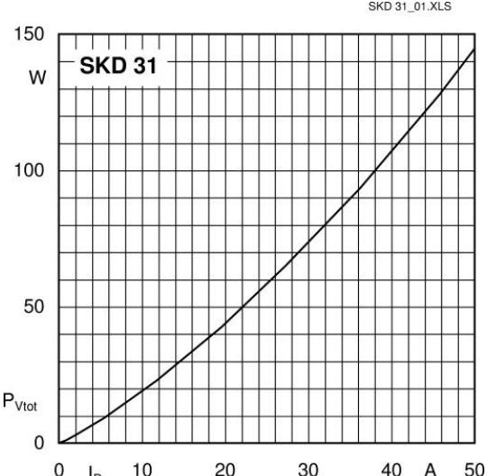
Fig. 3L Power dissipation vs. output current
