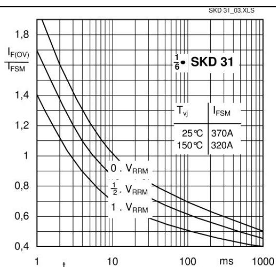
Fig. 6 Surge overload characteristics vs. time
