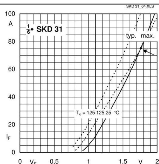
Fig. 9 Forward characteristics of a diode arm
