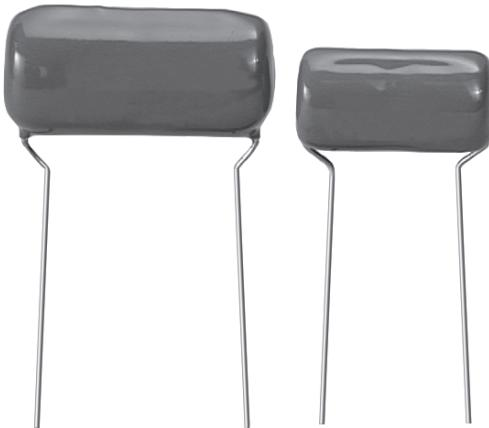
Polypropylene plastic film is employed as the dielectric in Type 715P ORANGE DROP® capacitors. Type 715P capacitors are ideal for applications where high AC current flow is found, as in certain solid-state TV vertical circuits, r-f generators and pulse-forming networks where dielectric heating is often a problem.
