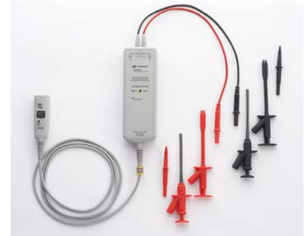
N2790A 100 MHz high voltage differential probe
