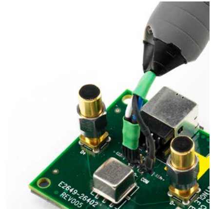
N2750A with N4822A socketed tip for application fixtures
