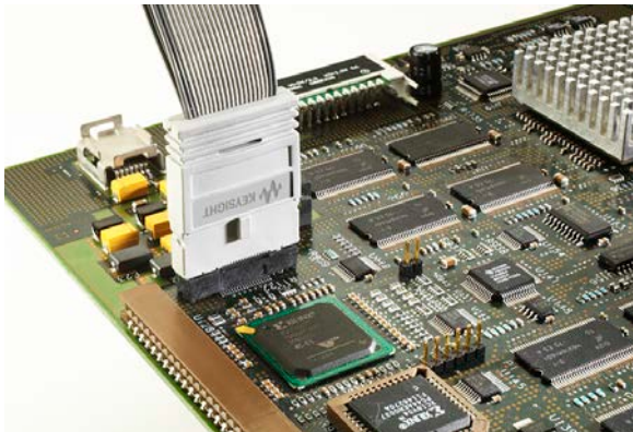
E5346A 34-channel Mictor connector probe
