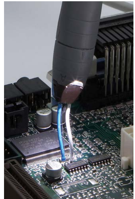
N2750A with solder-in tip
