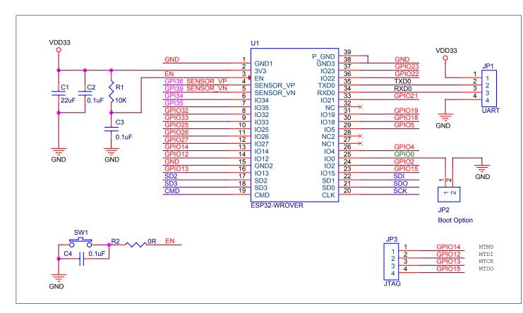
Figure 4: Peripheral Schematics of ESP32-WROVER
