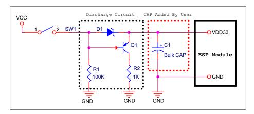
Figure 5: Discharge Circuit for VDD33 Rail
