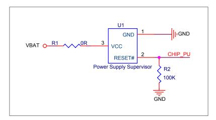
Figure 6: Reset Circuit
