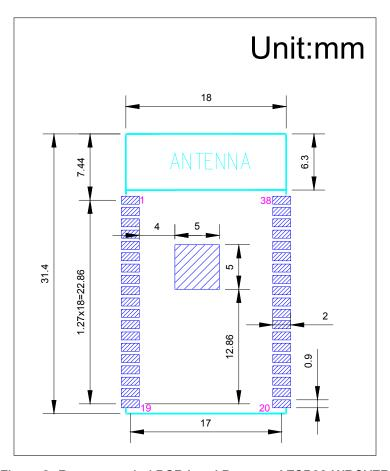
Figure 8: Recommended PCB Land Pattern of ESP32-WROVER
