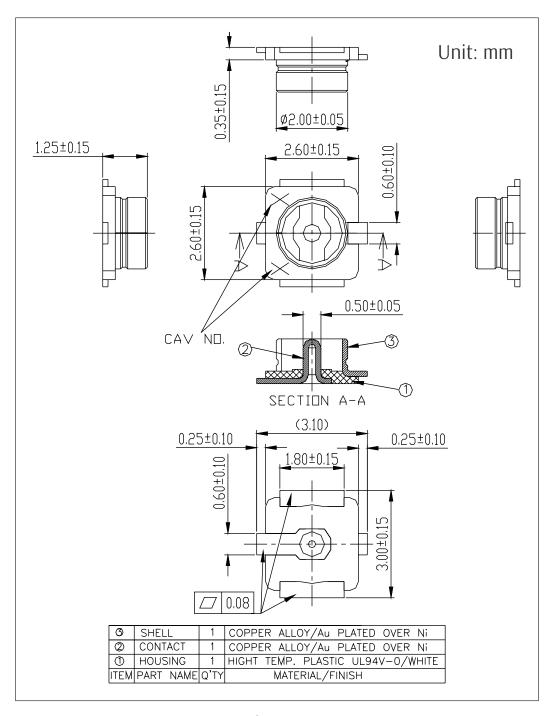
Figure 9: U.FL Connector Dimensions
