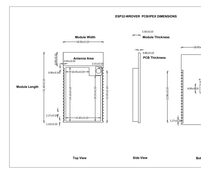
Figure 7: Physical Dimensions of ESP32-WROVER
