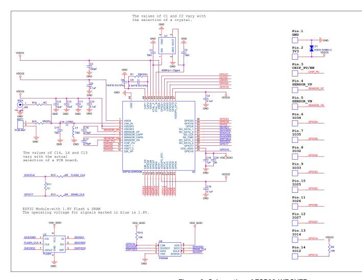
Figure 3: Schematics of ESP32-WROVER
