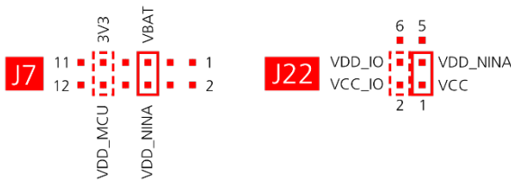
Figure 7: Jumper positions for battery powered operation, two jumpers are optional
