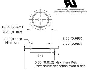
0.03 (0.001) Minimum Ref. (Applies to top edge of gasket or edge of crimp, whichever is higher.)
