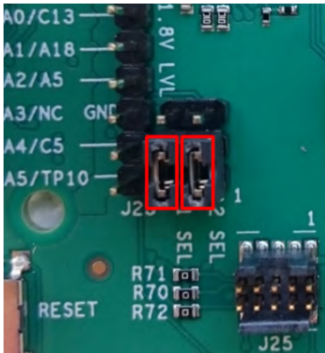
Figure 6: A1 and A2 as digital I/O on J2
