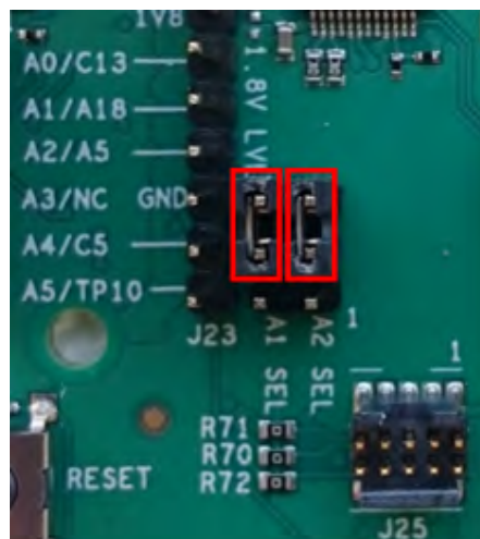
Figure 7: A1 and A2 as analog in on J2
