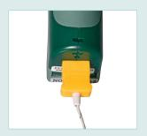
Type K input for contact measurements
