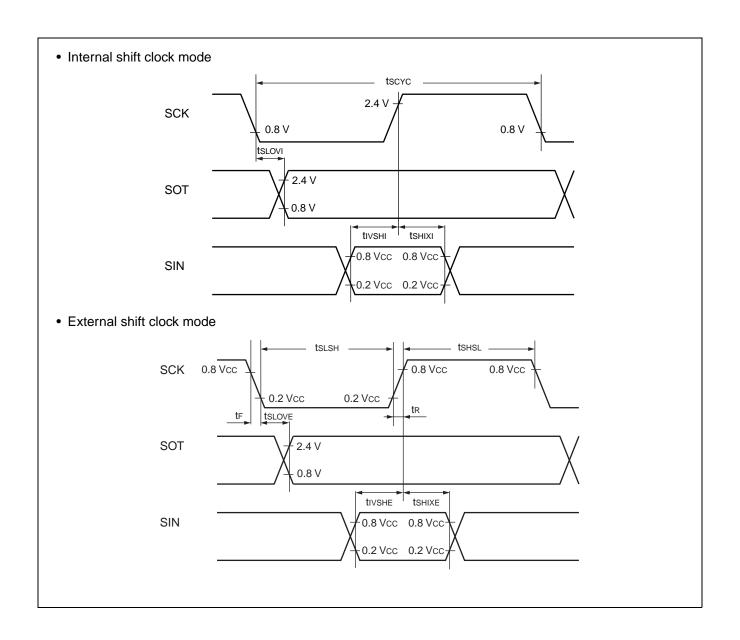
Sampling at the falling edge of sampling clock\*1 and prohibited serial clock delay\*2
