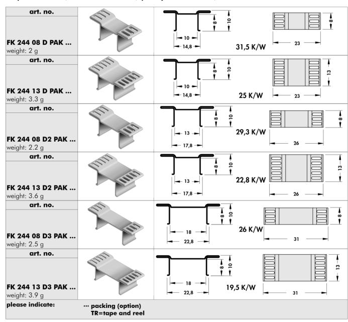
material: copper (Cu) material thickness: 0.6 mm surface treatment: solderable
