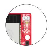
**CLOUD** LED turns on when your FLUO WI-FI is connected to the Internet
