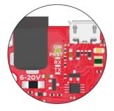
**ON** LED turns on when the FLUO WI-FI is powered up
