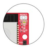
**STATUS** LED turns on when the firmware is running
