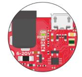
**PRST** LED turns on when both the ATmega644p and the ESP-32 have successfully rebooted.
