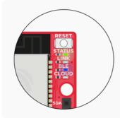
**BLE** LED blinks when the Bluetooth connection on your FLUO WI-FI is in discoverable mode
