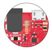
**RX/TX** LEDs flash when there is serial (USB Serial) data being transmitted to or from your FLUO WI-FI via the USB connection.
