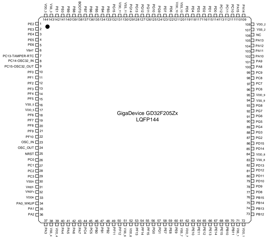
Figure 2. GD32F205Zx LQFP144 pinouts
