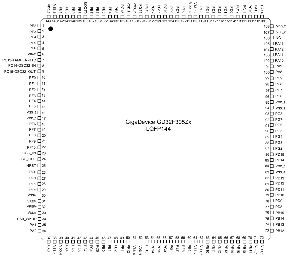
Figure 2. GD32F305Zx LQFP144 pinouts
