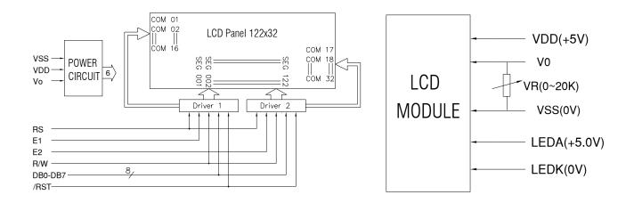
Figure 1. Block diagram
