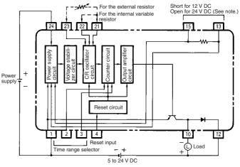
10: Solid-state output terminal 12: Terminal for the internal load surge absorbing diode **Note:** When using 12/24 V DC-operated models.
