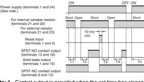
Note: 1. Control output is provided when the set time has elapsed  $(T_1 + T_2 \text{ or } T_3 + T_4).$
