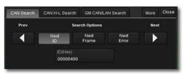
Search through long records of decoded data by entering specific message or frame details.
