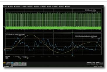
Here, information on the steering angle and steering angle rate of change is extracted from the CAN message acquisition, rescaled to decimal values, and plotted as a time-correlated "Track"
