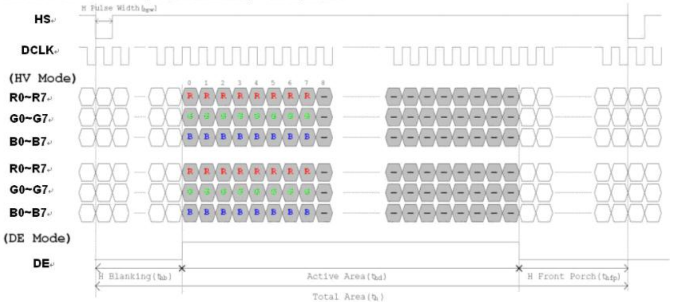
Horizontal input timing diagram.
