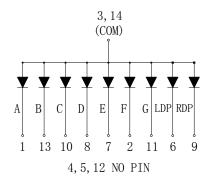
Internal Circuit Diagram (Common Cathode)
