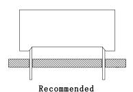
3. The component shall be placed at least 5mm from edge of PCB to avoid damage caused excessive heat during wave soldering.
