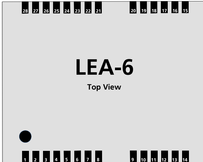
Figure 2 LEA-6 Pin Assignment
