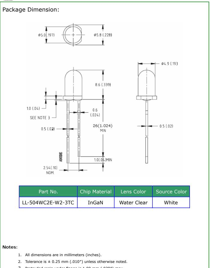
3. Protruded resin under flange is 1.00 mm (.039") max.
