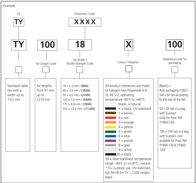
Note: Nylon (Polyamide) is inherently susceptible to environmental conditions. Ty-Fast® cable ties are moisturised to optimum performance levels at machineside and should be stored in cool dry areas out of direct sunlight. Cable ties are packaged in plastic bags to contain moisture and should remain sealed until ready for use.
