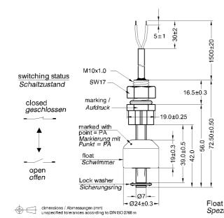
Material stem- polyamid black nut- polyamid black float- polyamid white lock washer- polyamid black O-ring- nitril caoutchouc black
