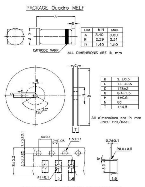
Accumulated pitch tolerance is  $\pm 0.2~\text{mm}$  over 1D pitches 8-mm Carrier tape for Quadro MELF - LS34 PACKAGE All dimensions are in mm
