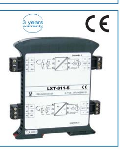
The LXT-811-S transducer converts temperature from an input sensor to the output current signal 4...20mA. A device works as a current loop regulator with galvanic separation between an input sensor and the output. The LXT-811-S is self powered from the current loop.
