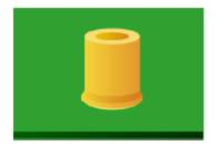
Solder the Mounting Pillar in place using standard surface mount Techniques
