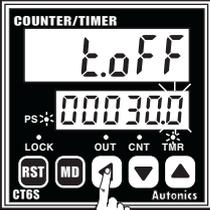
Advance to setting time change mode by press **MD** key. Shift the flashing digit to position "3" by press **←** key twice. (PS LED ON)
