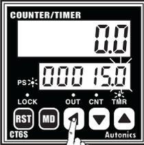
Advance to setting time change mode by press **MD** key. Shift the second digit to position "5" by press **←** key once. (PS LED ON)
