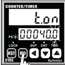
Press **MD** key to complete t.oFF time set and advance to t.on setting time change mode.
