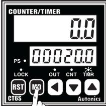
Press **MD** key to complete setting time change and return to timer RUN mode. (PS LED OFF)
