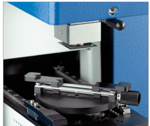
PBGA being held by Vacuum pik during Alignment procedure
