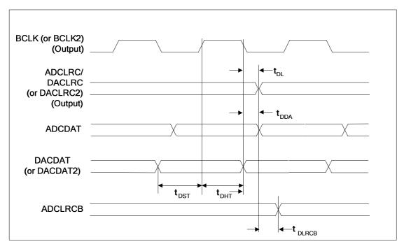
Figure 5 Digital Audio Data Timing - Master Mode (see Control Interface)
