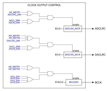
Figure 78 Clock Output Control
