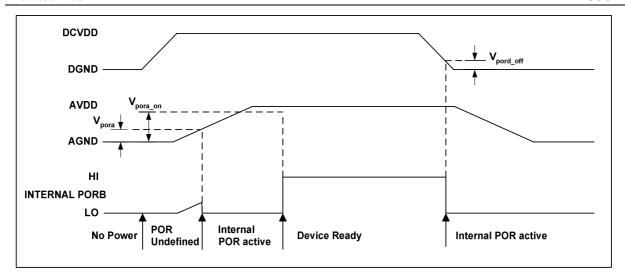
Figure 15 Typical Power up Sequence where DCVDD is powered before AVDD
