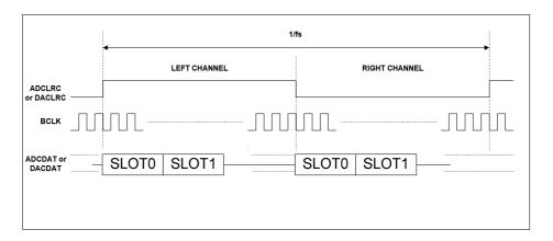
Figure 74 TDM in Left-Justified Mode
