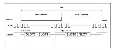
Figure 75 TDM in I<sup>2</sup>S Mode
