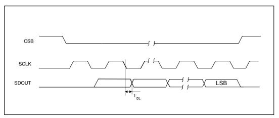
Figure 10 Control Interface Timing - 3-Wire Serial Control Mode (Read Cycle)
