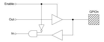
Figure 45 GPIO Pad
