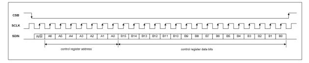
Figure 86 3-Wire Serial Control Interface
