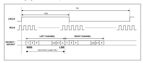
Figure 69 DSP Mode Audio Interface (mode A, AIF\_LRCLK\_INV=0, Master)
