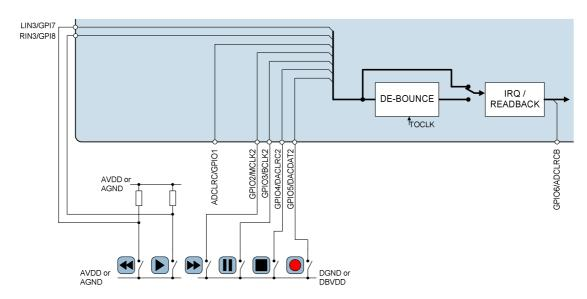
Figure 43 Example of Button Control Using GPIO Pins
