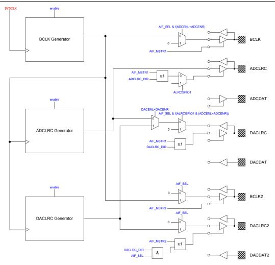
Figure 62 Audio Interface Output Control
