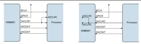
Figure 53 Master Mode with ADCLRC as GPIO Figure 54 Slave Mode with ADCLRC as GPIO
