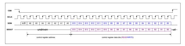
Figure 88 4-Wire Readback (wired-OR)
