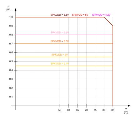
Figure 2 Class D Speaker Power De-Rating Curve
