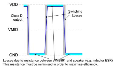
Figure 105 Speaker Connection Losses
