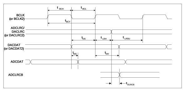
Figure 6 Digital Audio Data Timing - Slave Mode
