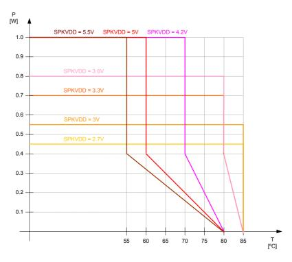
Figure 3 Class AB Speaker Power De-Rating Curve
