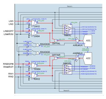
Figure 27 Differential Mode Signal Paths
