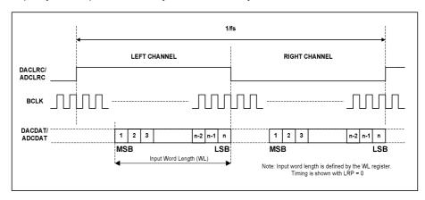
Figure 66 Right Justified Audio Interface (assuming n-bit word length)
