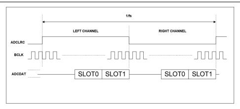
Figure 73 TDM in Right-Justified Mode
