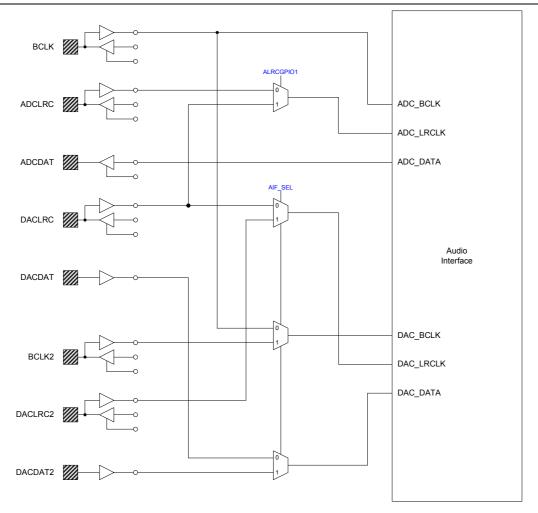
Figure 61 Audio Interface Input Flow
