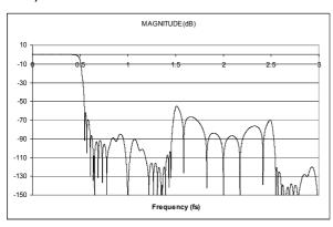
Figure 95 DAC Digital Filter Ripple (Normal Mode)
