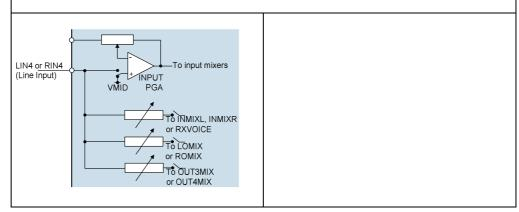
Figure 24 LIN4 or RIN4 as Line Inputs
