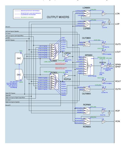
Figure 30 Control Registers for Output Signal Path
