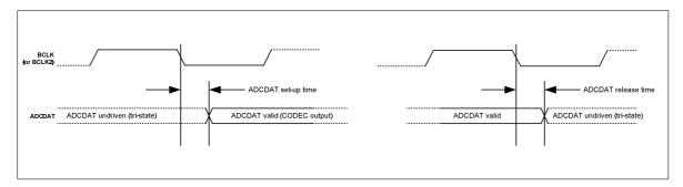
Figure 7 Digital Audio Data Timing - TDM Mode
