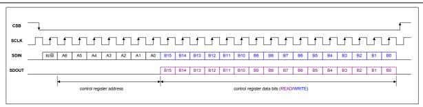
Figure 87 4-Wire Readback (Push 0/1)
