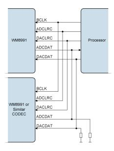
Figure 65 TDM with Processor as Master
