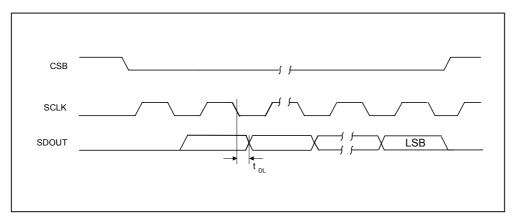
Figure 12 Control Interface Timing – 4-Wire Serial Control Mode (Read Cycle)
