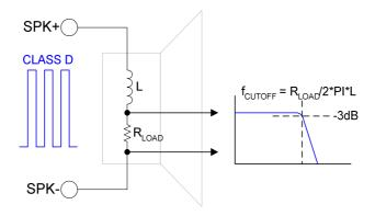
Figure 104 Speaker Equivalent Circuit
