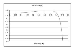
Figure 96 DAC Digital Filter Frequency Response (Sloping Stopband Mode)
