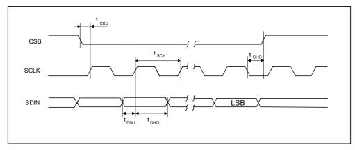
Figure 11 Control Interface Timing – 4-Wire Serial Control Mode (Write Cycle)
