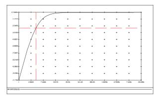
Figure 92 ADC Digital High Pass Filter Frequency Response (48kHz, Hi-Fi Mode, ADC\_HPF\_CUT[1:0]=00)
