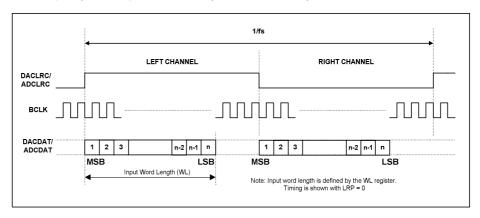
Figure 67 Left Justified Audio Interface (assuming n-bit word length)
