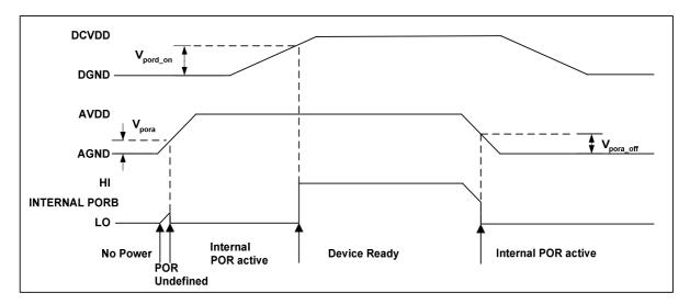
Figure 14 Typical Power up Sequence where AVDD is Powered before DCVDD
