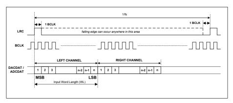
Figure 72 DSP Mode Audio Interface (mode B, AIF\_LRCLK\_INV=1, Slave)
