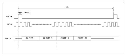
Figure 76 TDM in DSP Mode A
