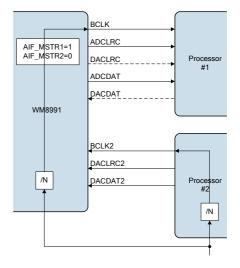
Figure 58 Interface 1 = Master, Interface 2 = Slave
