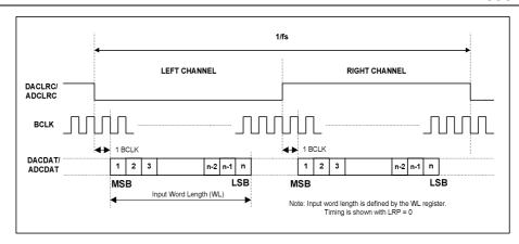
Figure 68 I2S Justified Audio Interface (assuming n-bit word length)
