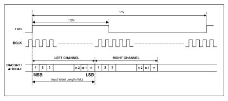
Figure 70 DSP Mode Audio Interface (mode B, AIF\_LRCLK\_INV=1, Master)
