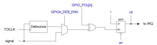
Figure 46 GPIO Function
