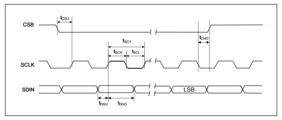
Figure 9 Control Interface Timing – 3-Wire Serial Control Mode (Write Cycle)
