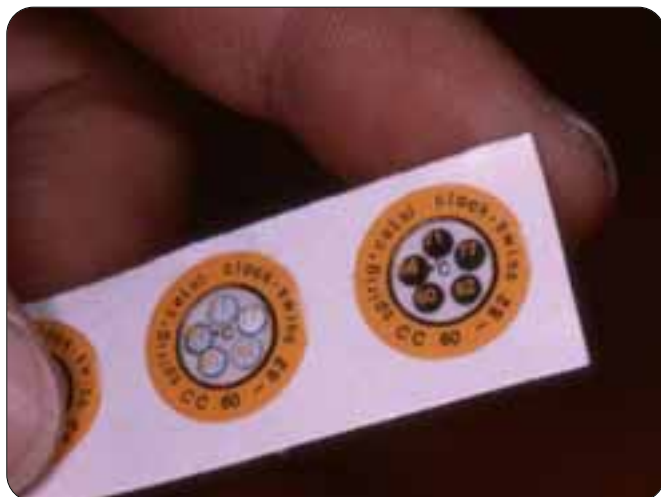
CelsiClock® with 5 temperature levels. CelsiClock®'s are also available with other temperature values and arrangements.
