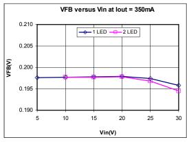
Fig. 6: Feedback Voltage vs Input Voltage
