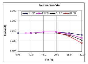
Fig. 5: Output Current vs Input Voltage
