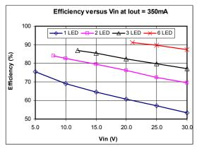
Fig. 4: Efficiency vs Input Voltage
