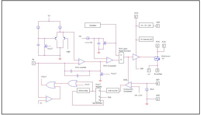
Fig. 2: XRP7603 Block Diagram
