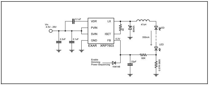
Fig. 1: XRP7603 Application Diagram
