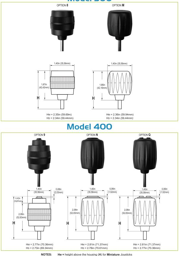
HM = height above the housing (H) for Miniature Joysticks Hs = height above the housing (H) for Standard Joysticks The drawings are not to scale, but are proportional.
