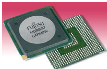
The Carmine GDC is the first device of its kind to be fabricated in 90nm technology.
