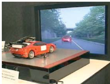
FlexRay, gyro and 32-bit microcontroller demonstration, combine to provide electronic stability control.
