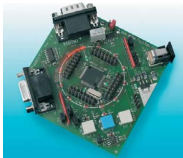
The MB91F267, offers three-phase motor control.
