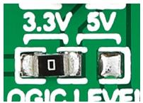
RF Meter click has an SMD jumper (zero ohm resistor) for setting the logic level either at 3.3V or 5V.
