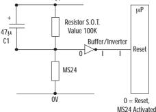
(logic 0) with no disturbance, a charge is permanently held in CI. With movement the MS24 goes momentarily open circuit allowing the charged capacitor to be seen at the inverter input which would change state giving a pulse to reset.
