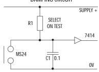
The output of the MS24 may be damped when less sensitivity is required by using a Schmitt trigger device as shown. Lowering the value of R1 (100 ohm min) will reduce the sensitivity of the switch
