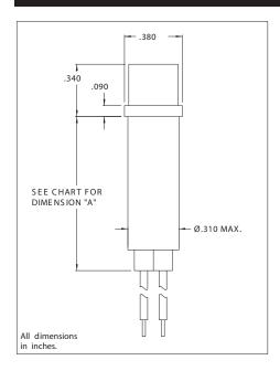
Mounting: Ø.310 MIN., supplied with push-on speednut SN1287.
