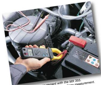
Battery current measurement with the MX 355. This can also be completed by DC voltage measurement.
