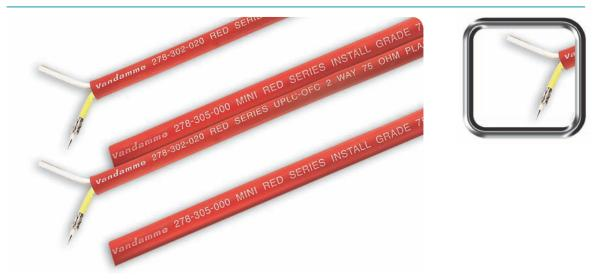
This range features Low Smoke Zero Halogen (LSZH) jacketed versions of the 2 and 5 way Red Series Miniature Video multicore. Mechanically and electrically identical, the use of LSZH materials makes them suitable for installations in public buildings and other situations where LSZH is specified.
