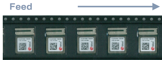
Figure 13: Orientation of NINA-B112 modules on tape
