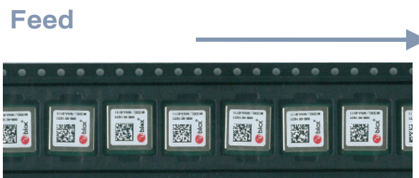
Figure 12: Orientation of NINA-B111 modules on tape
