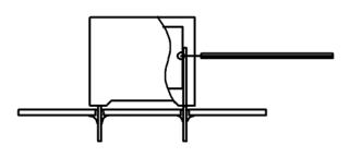
Temperature monitored inside the capacitor.
