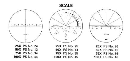
A scale is built into the scale chamber above the focusing ring. This scale can be easily interchanged according to use. Three kinds of scales—standard, for tools, for printing—are available. Specially designed scale can also be made to order.
