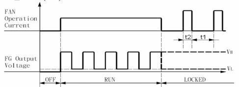
★Electrical Characteristics : (at  $Ta = 25^{\circ}C$ , Vcc = 12VDC)
