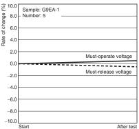
Characteristics were measured after applying a shock of 490 m²/s to the test piece 3 times each in 6 directions along 3 axes. The percentage rate of change is the average value for all of the samples.
