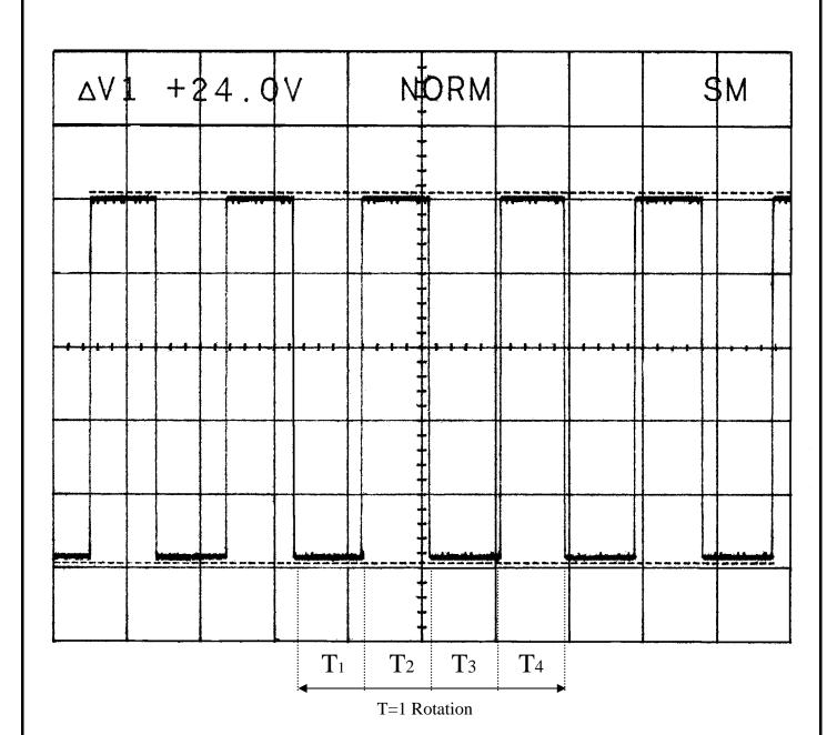
T=T1+T2+T3+T4 =(1 Rotation) T1=T2=T3=T4= $\frac{60}{4 \times \text{rpm}}$
