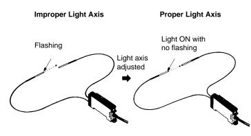
3. Set the mode selector to L-ON or D-ON after the light axis is adjusted.
