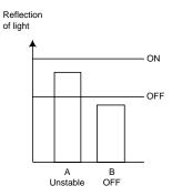
Reduce the sensitivity of the E3X with the sensitivity adjuster and turn off zone B.
