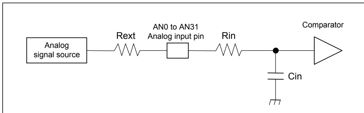
(Equation 1)  $T_s \geq (R_{in} + R_{ext}) \times C_{in} \times 9$
